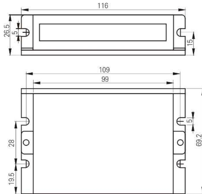
Figure 1: Mechanical specifications
